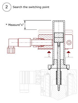
Slightly move the clamping plate upwards until the limit switch contact 1-3 is closed. Then move the clamping plate 5 mm upwards.
