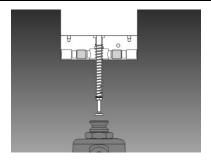
• Fasten the positioner using the two stud bolts.
